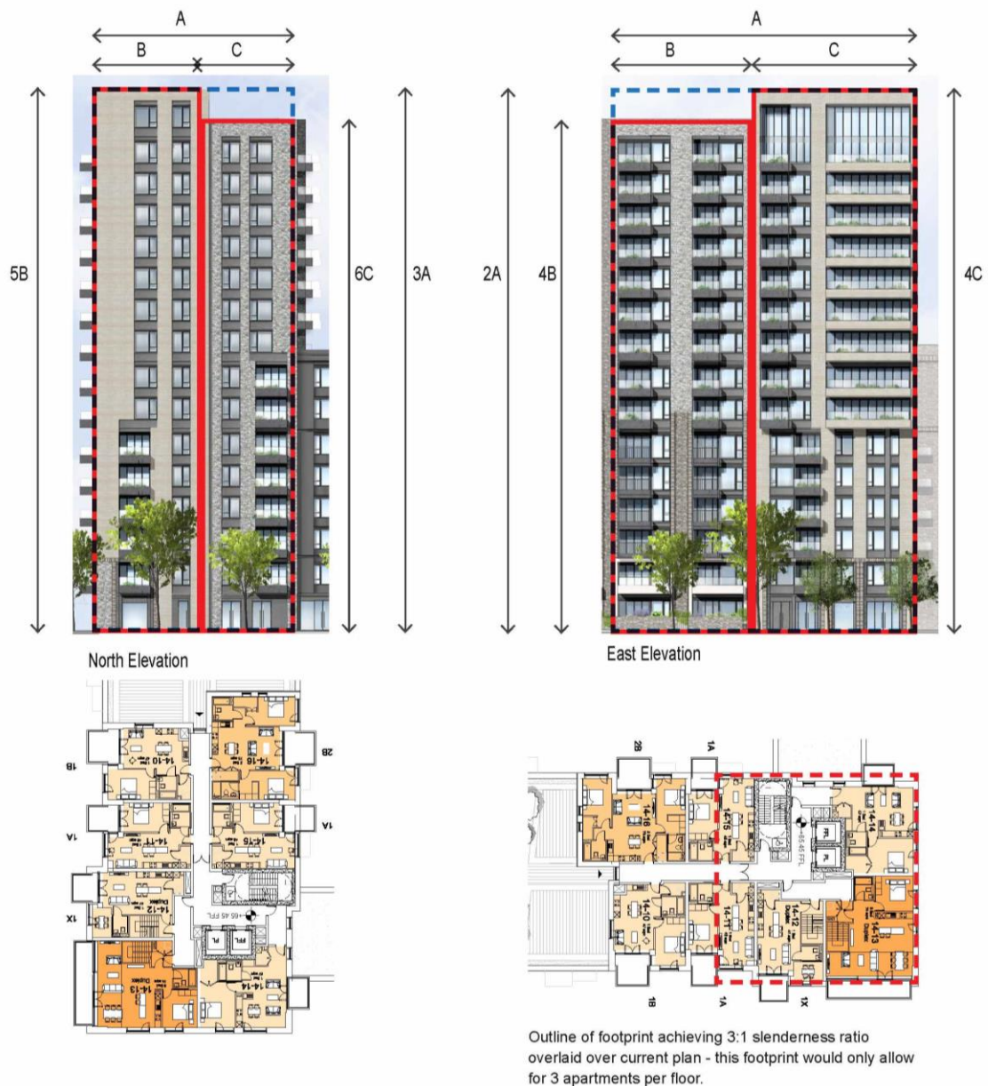
FIGURE 35 PROPOSED TOWER 1, NORTH AND EAST ELEVATION AND LAYOUT PLANS SHOWING TOWER SLENDERNESS
